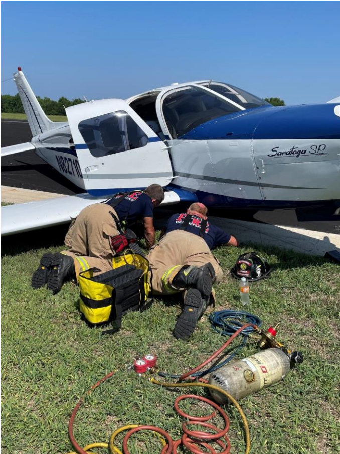
Pictured Below: Captain Jon Moore and Driver Robert Haggard use airbags to lift the wing of an airplane after the landing gear collapsed after landing.
